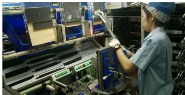
Figure B: The Simple Jig install for 3 size of part (The packing)
