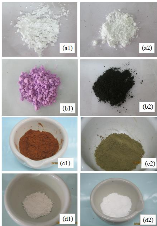
Figure 1. Precursors prepared by the chemical co-precipitation method and perovskite oxides after calcinations at 900 °C (LaAlO 3 ), 600 °C (LaCoO 3 ), 800 °C (LaFeO 3 ), and 1200 °C (LaGdO 3 ) for 2 h: (a1) LaAlO 3 precursor, (a2) LaAlO 3 perovskite, (b1) LaCoO 3 precursor, (b2) LaCoO 3 perovskite, (c1) LaFeO 3 precursor, (c2) LaFeO 3 perovskite, (d1) LaGdO 3 precursor, and (d2) LaGdO 3 perovskite.
