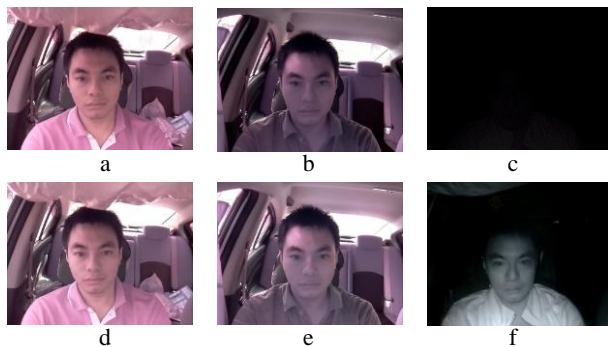
Figure 1. Faces captured without Infrared (IR) illumination in (a) bright, (b) dim, and (c) dark situations, and those with IR illumination in (d) bright, (e) dim, and (f) dark situations.
