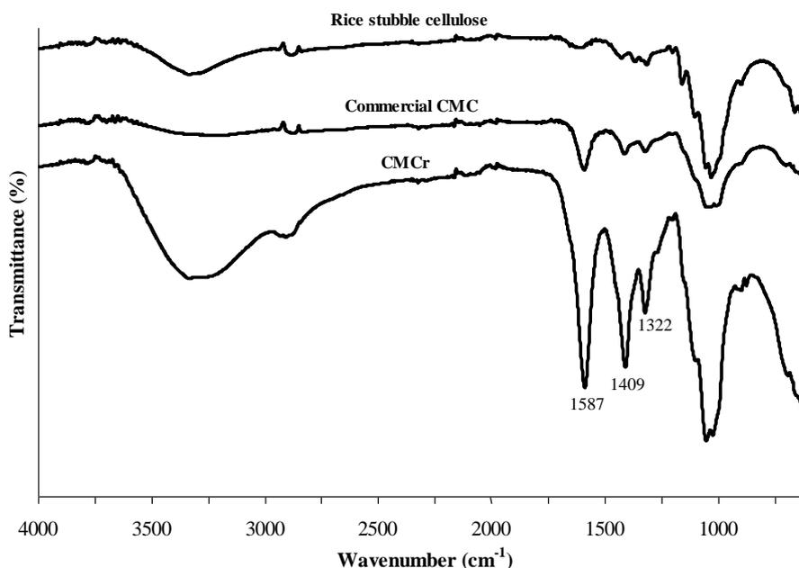
Figure 5. FTIR spectra of rice stubble cellulose, commercial carboxymethyl cellulose (CMC) and CMC from rice stubble cellulose using 7 g of chloroacetic acid per 5 g of rice stubble cellulose for 180 min at 50°C (CMCr).
