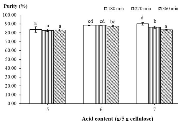
Figure 4. Effect of synthesis conditions (acid content and time) on purity of carboxymethyl cellulose from rice stubble. The same letters (a, b, c, d) were not statistically different ( $p < 0.05$ ).
