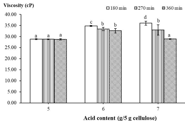
Figure 3. Effect of synthesis conditions (acid content and time) on viscosity of carboxymethyl cellulose from rice stubble. The same letters (a, b, c, d) were not statistically different (p < 0.05).
