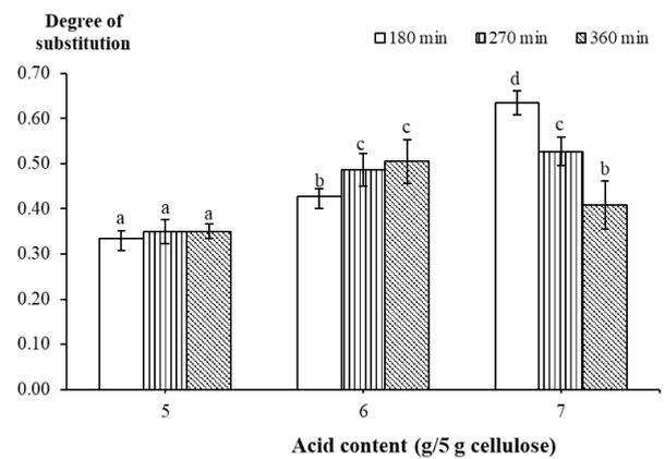
Figure 2. Effect of synthesis conditions (acid content and time) on degree of substitution (DS) of carboxymethyl cellulose from rice stubble. The same letters (a, b, c, d) were not statistically different (p < 0.05).
