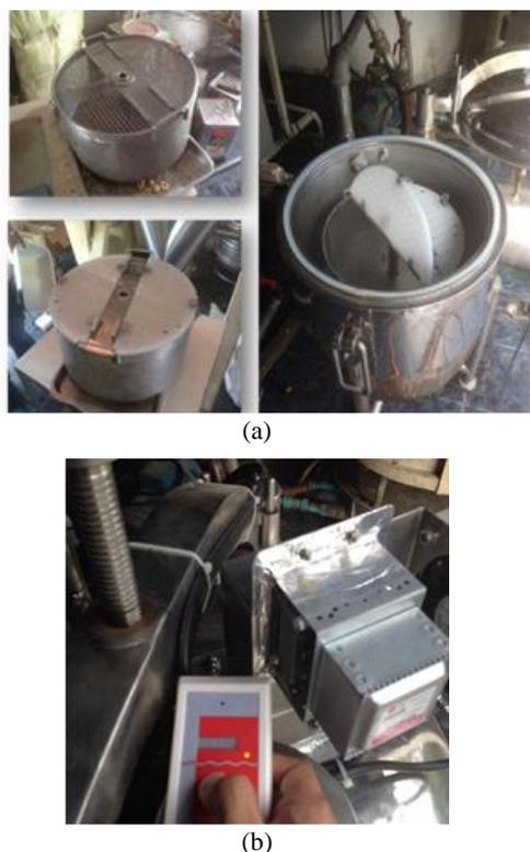
Figure 3. Modifications and safety of microwave vacuum frying machine: (a) Modification of frying basket lid using polypropylene and (b) Test of microwave leakage by RCME Microwave Leakage Detector. (RCME: Research Center of Microwave Utilization in Engineering, the Department of Mechanical Engineering, the Faculty of Engineering, Thammasat University)
