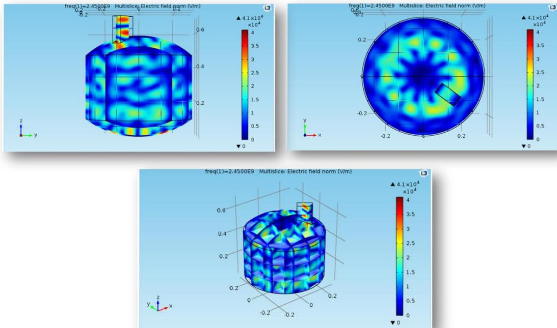
Figure 2. Optimized electromagnetic field simulation result of waveguide and cavity installation design from COMSOL Multiphysics Software Version 5.1.
