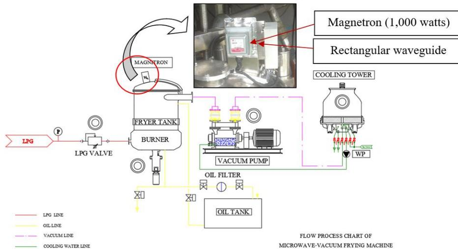
Figure 1. Conceptual design for the microwave vacuum frying machine.
