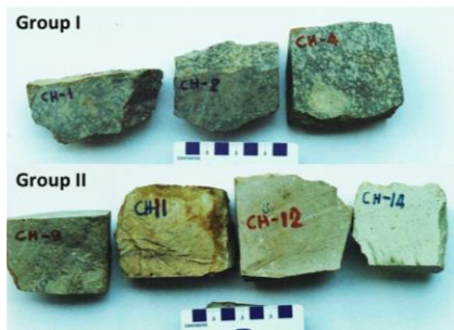
Figure 2. Photographs showing the studied volcanic rock samples (Chae Hom rhyolite) with different proportions of lighter-color and darker-color portions in Group I and Group II.
