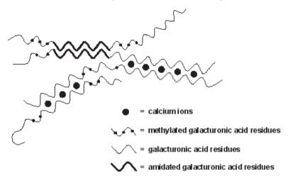
**Fig. 4** Model for the gelation of amidated LM-pectins showing ionic interactions between galacturonic acid residues and hydrogen bonding between amidated galacturonic acid residues (adapted from Sriamornsak, 2002).
