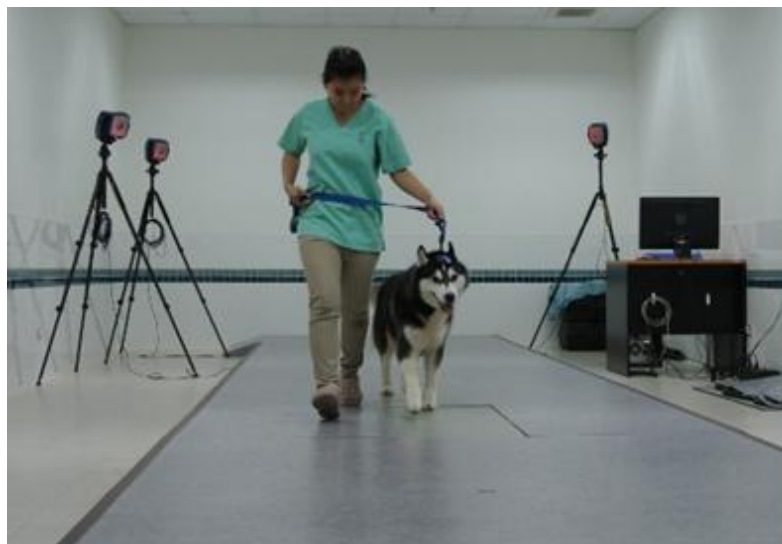
Figure 1 Measurement of PVF using force plate gait analysis
