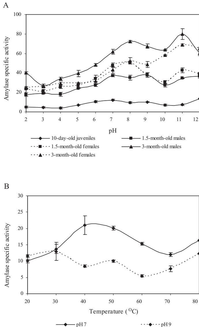
**Figure 1** Amylase specific activity ( $\mu\text{mol maltose h}^{-1} \text{mg protein}^{-1}$ ) at various stages of development of *B. splendens*: (A) pH profiles at ambient temperature; and (B) temperature profiles at optimal pH levels in 10-day-old juveniles.
