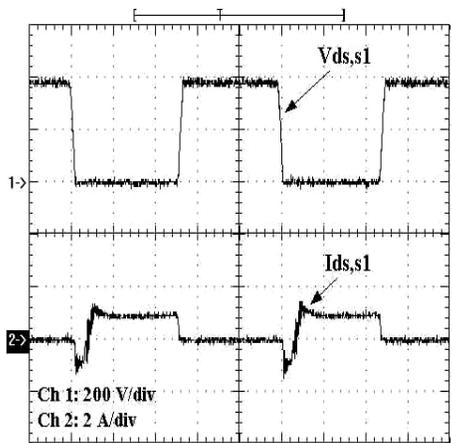
Fig. 10. Current and voltage waveforms of  $s_1$  for the proposed ZVT PWM boost PFC converter,  $t = 5\mu\text{s}/\text{div}$
