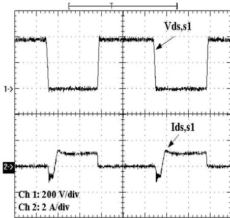
Fig. 9. Current and voltage waveforms of  $s_1$  for the conventional ZVT PWM boost PFC converter,  $t = 5\mu\text{s}/\text{div}$
