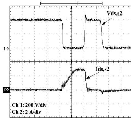
Fig. 11. Current and voltage waveforms of  $s_2$  for the conventional ZVT PWM boost PFC converter,  $t = 1\mu\text{s}/\text{div}$
