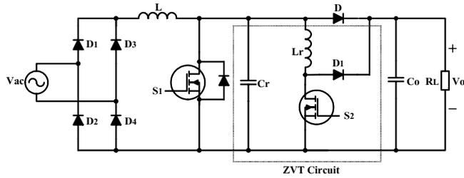
Fig. 1. Conventional ZVT PWM boost PFC converter
