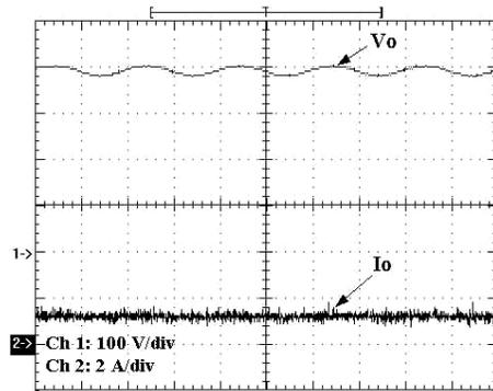
Fig. 8. Experimental results of the output voltage and current for the proposed ZVT PWM boost PFC converter,  $t = 5\text{ms/div}$
