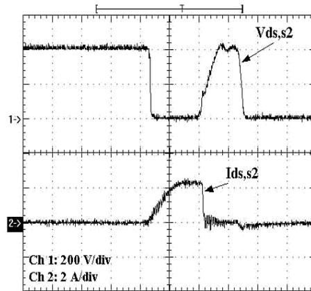
Fig. 12. Current and voltage waveforms of  $s_2$  for the proposed ZVT PWM boost PFC converter,  $t = 1\mu\text{s}/\text{div}$
