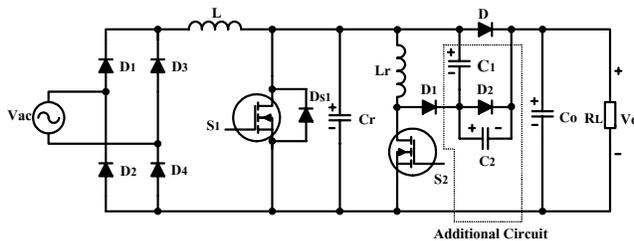
Fig. 2. Proposed ZVT PWM boost PFC converter
