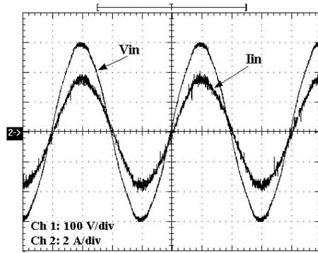
Fig. 7. Experimental results of the input voltage and current for the proposed ZVT PWM boost PFC converter,  $t = 5\text{ms/div}$
