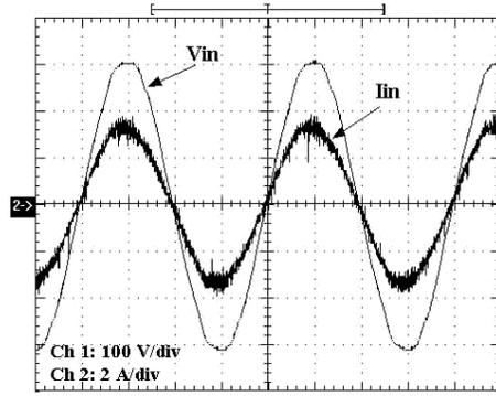
Fig. 6. Experimental results of the input voltage and current for the conventional ZVT PWM boost PFC converter,  $t = 5\text{ms/div}$
