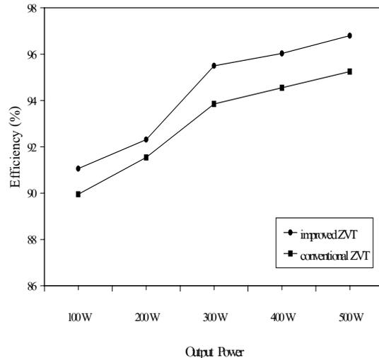
Fig. 13. Efficiency comparison between both converters
