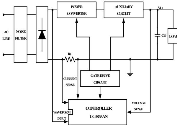
Fig. 5. Block diagram of an experimental circuit
