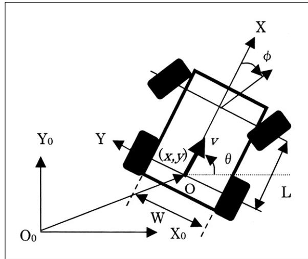
**Figure 3.** 4-Wheel Mobile Robot Model.
