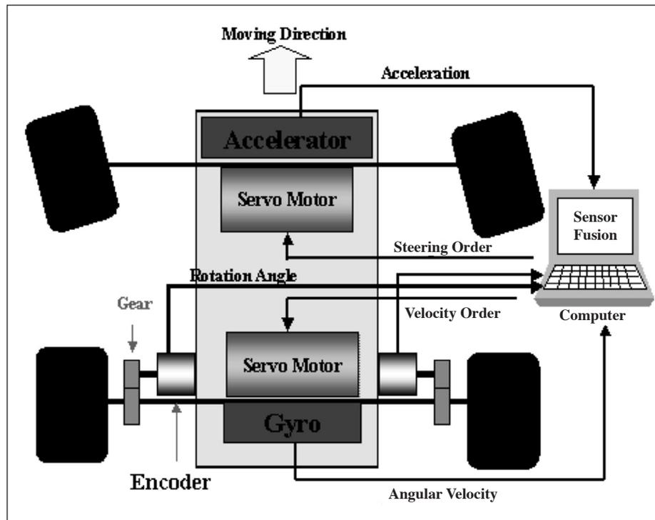
**Figure 5.** Structure of the Practical Mobile Robot.
