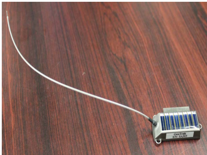
Fig. 2 The Argos signal sender. Main body includes solar battery on the back with long antenna.
