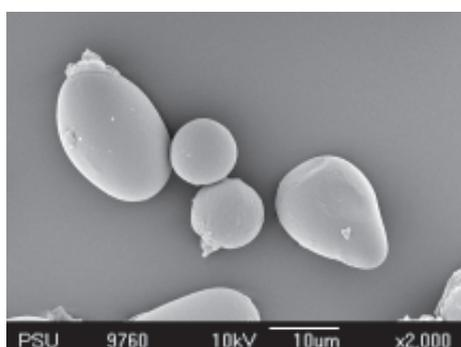
Figure 1. Scanning electron micrograph of starch granules from bambarra groundnut at magnification 2000X
