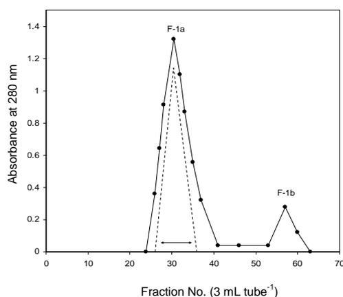
**Figure 2** Ion exchange chromatography of lipase enzyme on DEAE-cellulose. The enzyme solution (50 mg) was applied to the column (2.1x25 cm) pre-equilibrated with 10 mM Tris-HCl buffer, pH 8.4 at 4°C and eluted by a linear gradient of NaCl (0 to 0.3 M) in the same buffer. Flow rate: 25 mL h<sup>-1</sup>. Dashed line indicates lipase activity.
