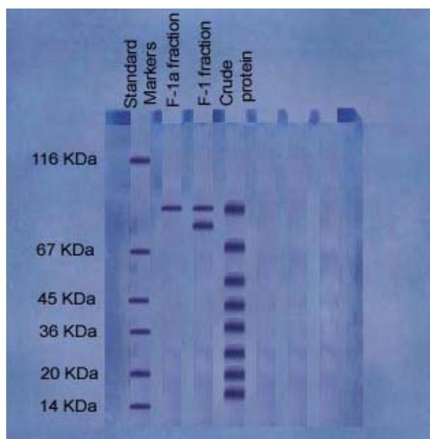
**Figure 3** Photographic representation of the SDS-PAGE (7.5% gel) of different fractions of fish lipase obtained during purification steps and standard proteins (Staining reagent 1% Amido black).
