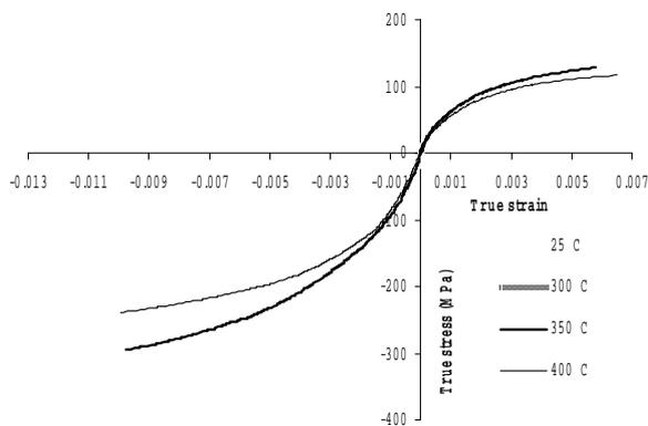
**Figure 7** True stress-true strain curves for Rover cast iron disc material
