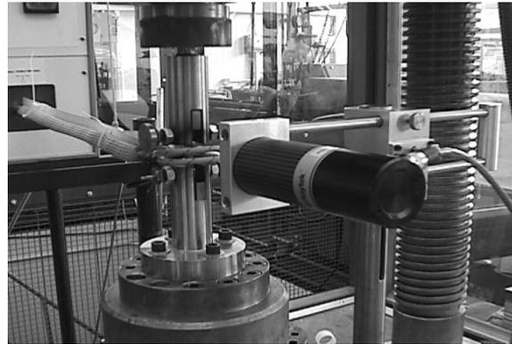
**Figure 2** Infrared detector and induction heating furnace
