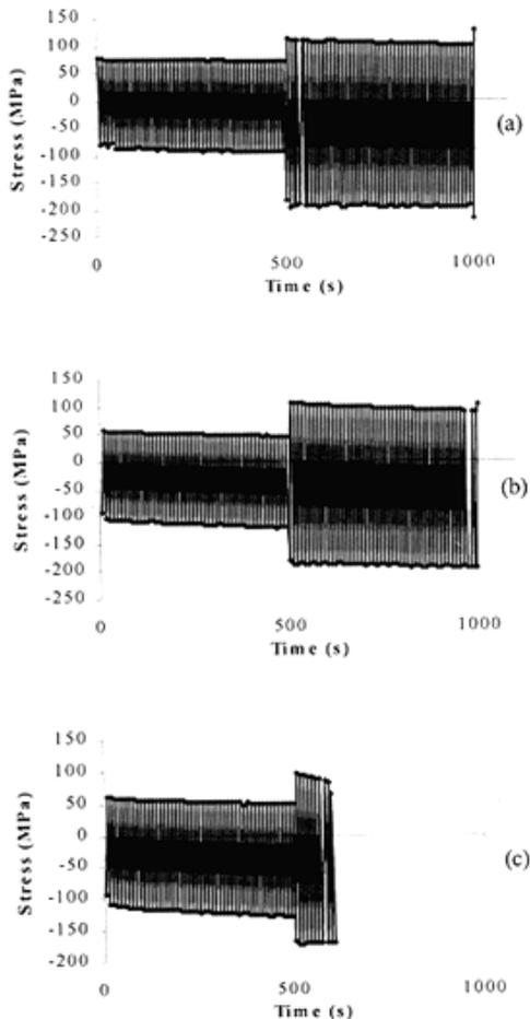
**Figure 9** True stress-time curves for Rover cast iron disc material at (a) room temperature, (b) 300°C, (c) 400°C
