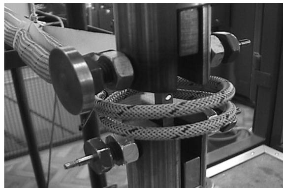
**Figure 3** Induction coil for high temperature testing
