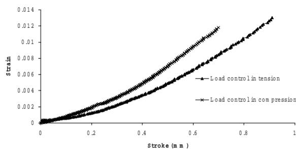
**Figure 6** Relation between the specimen strain and the crosshead for the load control
