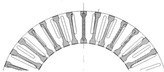
**Figure 1** Layout of specimens on the rubbing surface
