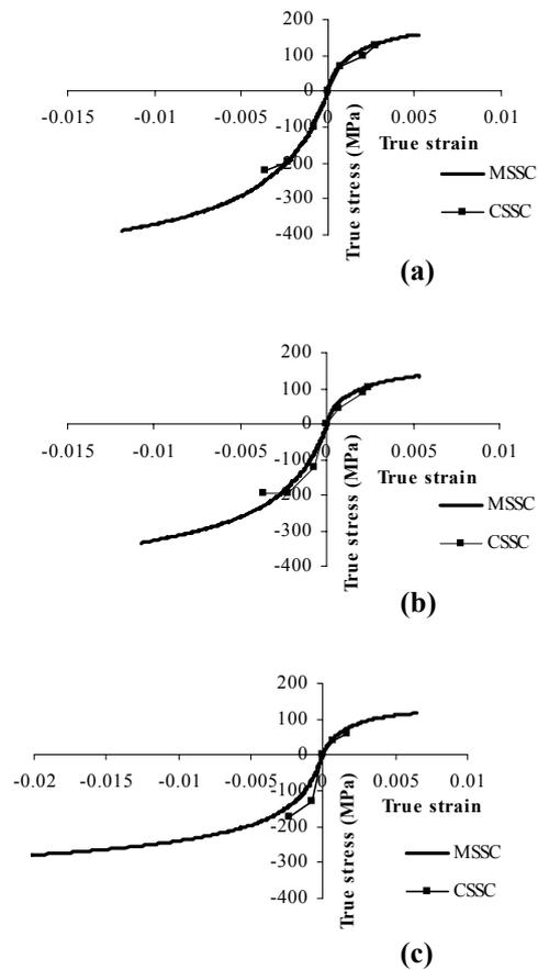
**Figure 10** Comparison between CSSC and MSSC at (a) room temperature, (b) 300°C, (c) 400°C
