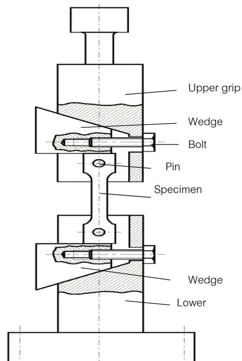
**Figure 4** Side view of grip assembly
