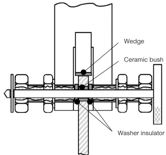
**Figure 5** Front view of grip assembly for elevated temperature
