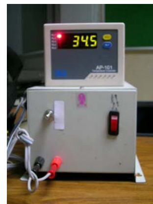
Figure 2 A temperature digital monitor showing an increase in thermal temperature with 0.5°C/sec increments and a control unit providing safety for cats from skin thermal stimulation by an automatic safety cut-off switch.
